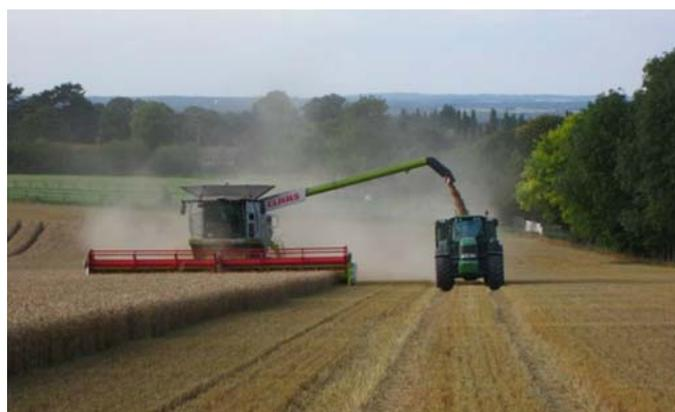
Extended combine auger allows harvest traffic to remain on CTF lanes
